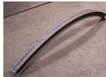
Cold bent specimen HE 100A (left) and residual stress measurements (right)
